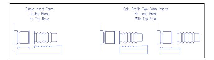
Specifically addressing the barbed fittings common to brass parts, caution is warranted when thin walls are produced in simultaneous drilling and forming operations. The combined heat may cause part cracking. Staggering operations can provide time for cooling the part. Voluminous as well as high pressure coolant can assist in heat dissipation and chip issues.
